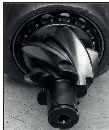
There are just 5 teeth on the RC drive pinion shaft vs. 7 on the WC. The end of the shaft is machined for a bearing but gets none.
