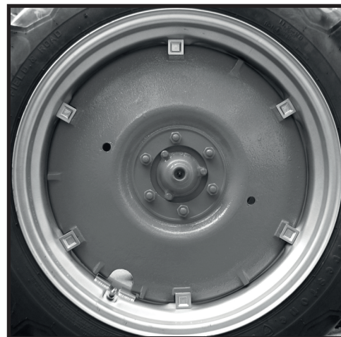
The RC wheel center had just one cut-out vs. two on the WC. We also see the special mounting bolts here.
