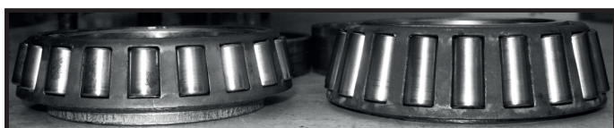
Final drive hub inner bearing cones. The RC used the smaller bearing on the left held out by a spacer. The WC used the larger bearing on the right.
